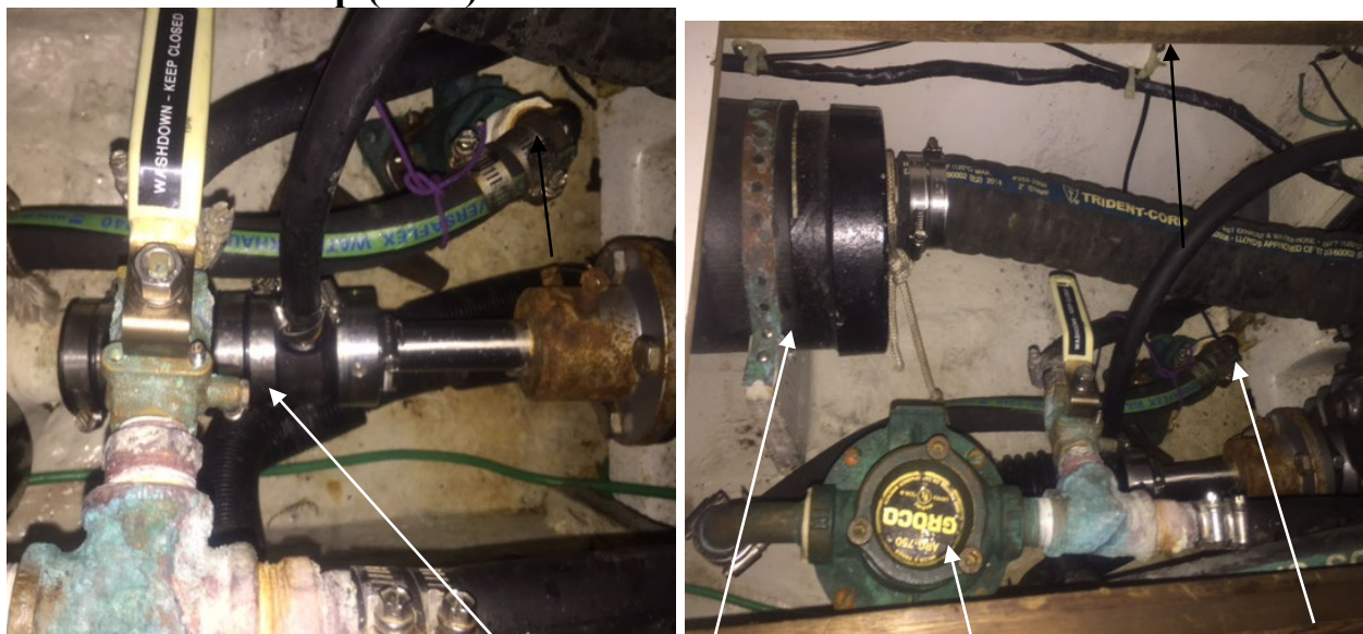
Washdown seacock/ Dripless shaft seal/ Muffler/exhaust/ Raw water strainer / Raw water intake
