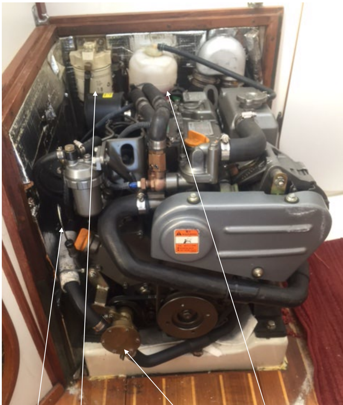
Oil Dipstick/ Fuel Filter/ Raw water impeller/ Fresh Water expansion tank
